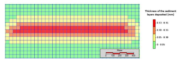
Figure 5: Seabed top view in the Case Study 1 transect region: simulated sediment layer deposited in the continental shelf by the double-rig trawling operation in Campos Basin.
