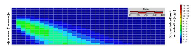
Figure 6. Simulated suspended sediment concentration from the single-rig trawling operation in the slope of the Campos Basin. Vertical cut along Case Study 2 transect.
