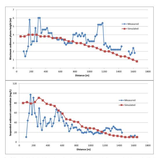
Figure 3. Measured and simulated longitudinal maximum sediment plume height (up) and suspended sediment concentrations in the water column (down) originated by the bottom travling operation (Mengual *et al.*, 2016).
