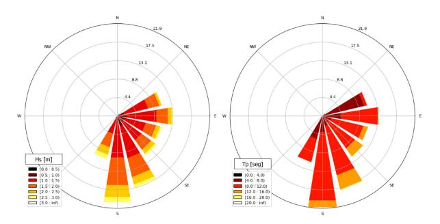
Figure 2. Wave roses for the significant wave height (Hs) [m] and peak wave period (Ts) [s]. Data calculated by Instituto Nacional del Agua (INA).
