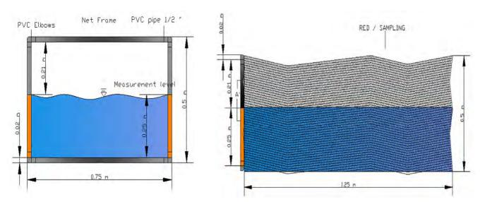
Figure 1 - Multifilament device diagram for sample collecting.
