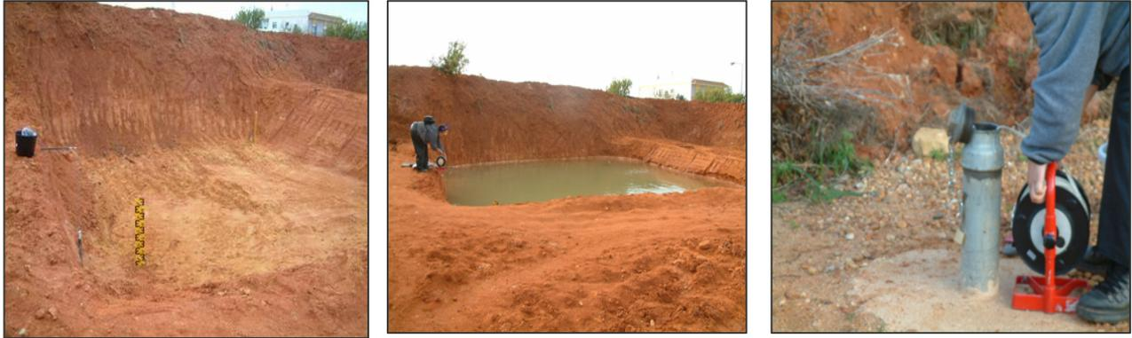
Figure 2 – Infiltration basin in the second layer and monitoring equipment used for the infiltration test.
