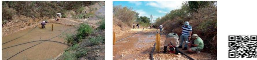
Figure 5-5: Rio Seco riverbed infiltration ponds (left image) and MAR clogging and infiltration experiments developed in Rio Seco (right image) (Campina de Faro, Algarve, Portugal). Illustrations from MARSOL. For more details on this MARSOL project click [here](#) or scan the QR code.
