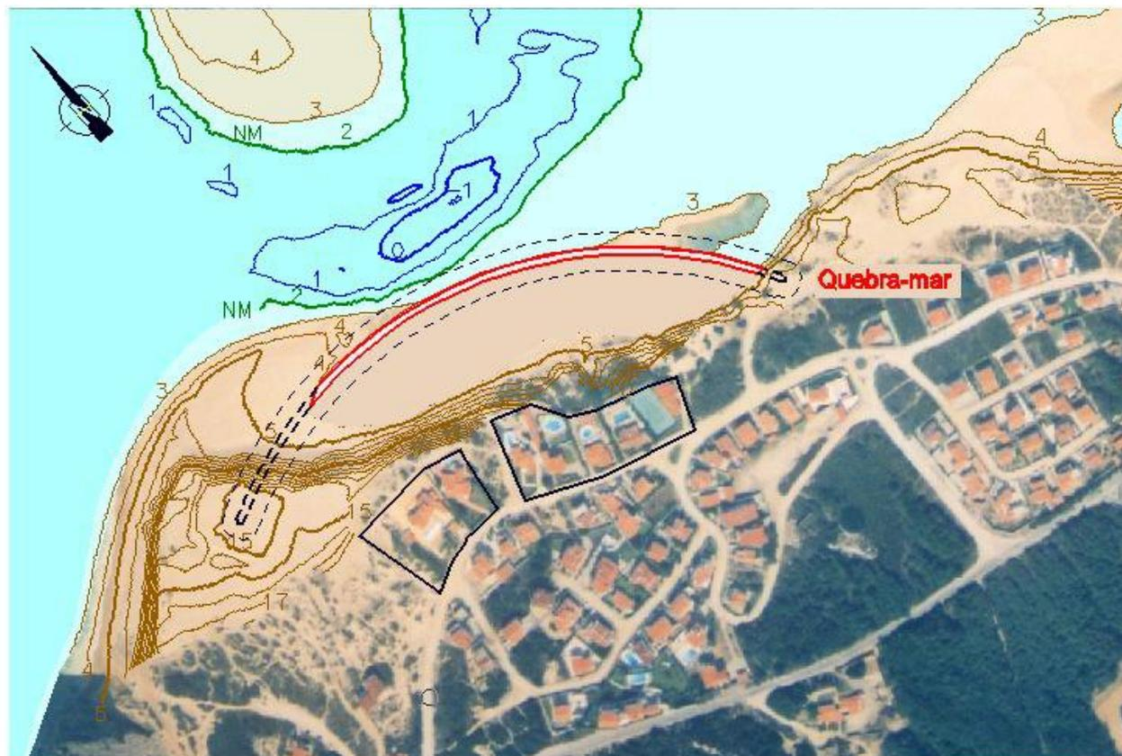
Figura 7 – Quebra-mar aderente à margem (in Clímaco, 2003). Sea-wall breakwater (from Clímaco, 2003).
