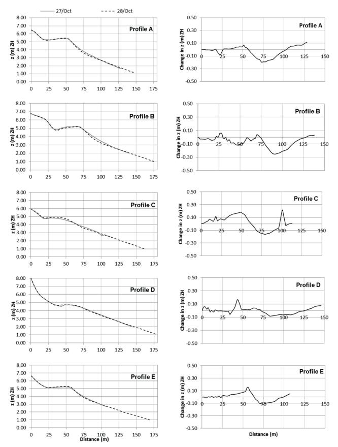
Figure 6. Morphological evolution of profiles A, B, C, D and E: profiles measured on the 27 and 28 of October (left column); and corresponding change in z (m) ( $<0 \Rightarrow$  erosion and  $>0 \Rightarrow$  accretion) (right column).
