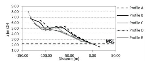
Figure 5. Cross-shore beach profiles A, B, C, D and E measured on the 27 of October. *Figura 5. Perfis transversais de praia A, B, C, D e E medidos em 27 de Outubro.*
