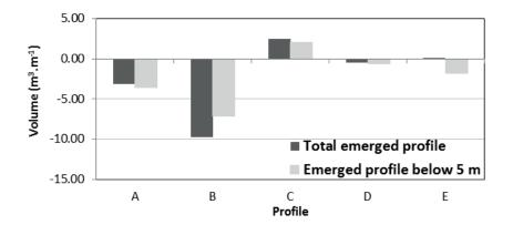
Figure 7. Change in volume in profiles A to E ( $<0 \Rightarrow$  erosion and  $>0 \Rightarrow$  accretion), for the total and the below 5 m ZH part of the emerged profiles.
