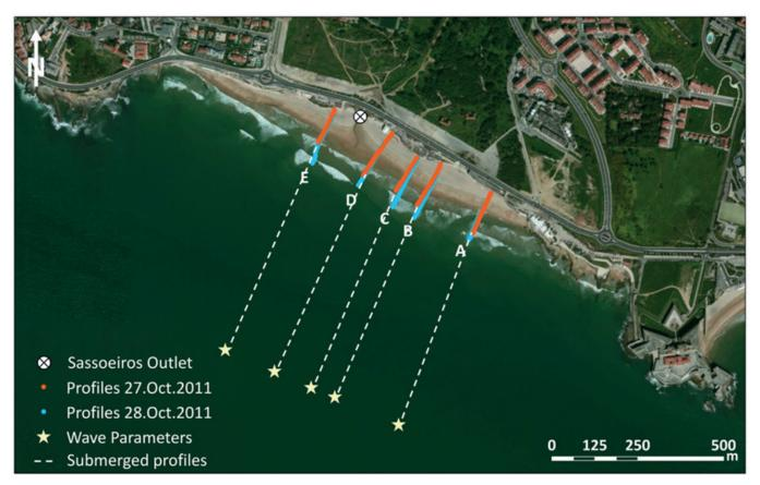
Figure 3. Location of the cross-shore profiles A, B, C, D and E surveyed on the 27 and 28 of October; position corresponding to the closure depth (10 m ZH) and to the wave parameters of each cross-shore profile; and location of the Sassoeiros stream outlet.
