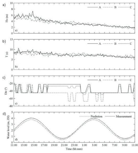
Figure 2 - Offshore wave parameters a) Hs, b) Tz and c) Dir relative to the geographic North (positive clockwise) in Sines (A), Leixões (B) and in front of the study area (C); and d) sea level at Cascais gauge during the study period.
