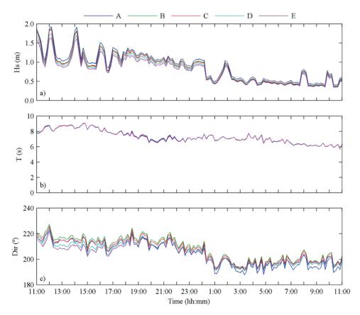
Figure 4 - Wave parameters Hs, Tz and Dir relative to the geographic North (positive clockwise) at the closure depth (10 m ZH) of profiles A, B, C, D and E during the study period.
