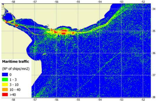
Figure 3 - Density map of vessel occurrences in Uruguayan waters represented as the accumulated daily presences of ships from June 2012 to July 2013 per cell (1.0nm side).
