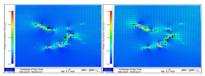
Figure 13 - Tidal currents in the archipelago of Cape Verde (maximum velocity 0.3 m/s) during ebb and flooding (20<sup>th</sup> May 2000).
