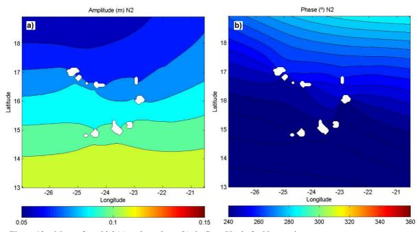
Figure 12 – Maps of co-tidal (a) and co-phase (b) in Cape Verde for N<sub>2</sub> constituent.
