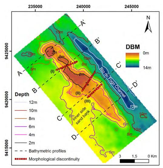
Figure 2 - D*igital Bathymetric Models* (DBM) interpolated from the Empirical Baeysian Kriging (EBK). The positions of the selected bathymetric profiles are located in dash lines (see Figure 4). (I), (II) and (III) morphological discontinuities are observed.
