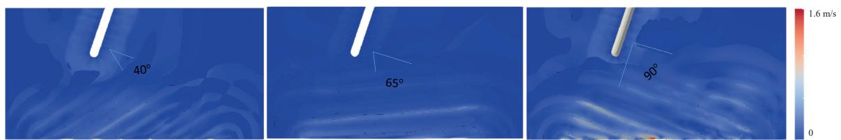
Figure 4: Snapshots of the numerical simulations, showing velocity magnitude (0 to 1.6 m/s) on free-surface and around the breakwater for incident irregular wave train angle at  $t=6$  for: a)  $40^\circ$ : T13; b)  $65^\circ$ : T19; and c)  $90^\circ$ : T25.
