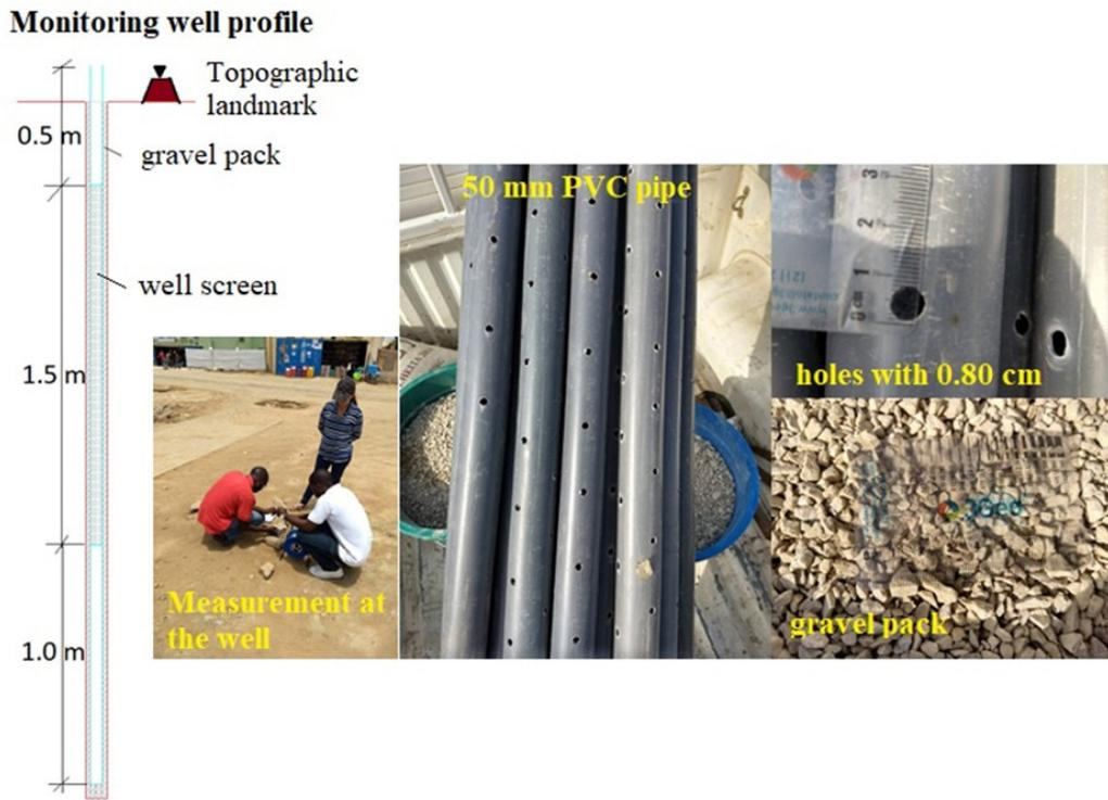
Figure 7. General profile of the monitoring wells.
