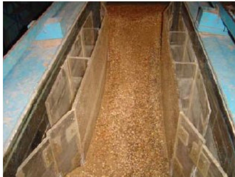
Fig. 6.45 Photograph showing equilibrium scour within a long contraction with a thin gravel-layer
